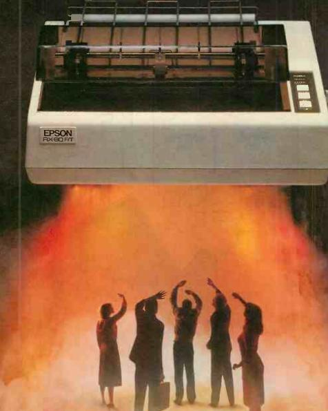
Epson have done it again! Realising a genuine need in the market place for a printer that not only has the same advanced features as its sister, the well tested RX-80, but also has the ability to accept both single sheet and fanfold paper; we bring you the RX-80 F/T.
